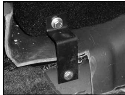
STEP 26 Secure the bottom of the Stealthbox® using the factory bolt.
